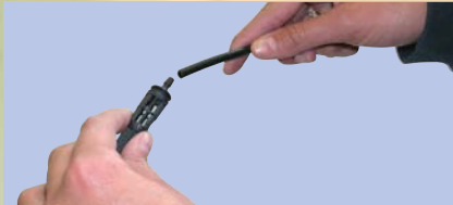
a. Fit drippers to dripper line
