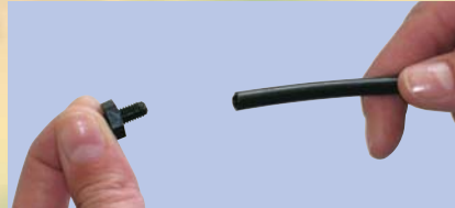
b. Screw threaded nipples into end of dripper line
